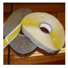
Figure 3 - Air Sealant Tape
