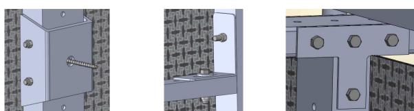
Figure 4 – Brackets & Wall Anchor
